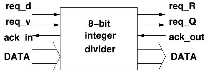
Figure 1: Lab 4 integer divider block diagram.
